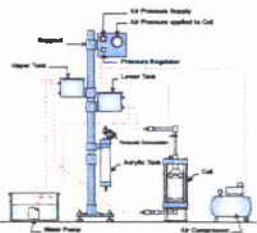
Purpose : To determine longitudinal flow properties of PVD
